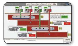
This system controls the loading of aggregate into rail cars. The operator has full control of the reclaim system, as well as the loading of each railcar, in automatic or manual modes of operation. KSS' **BatchMaster®** software is utilized as the loading manifest for weighing, invoicing, and shipping records.
