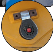
Rear Load Pin and Beam Load Cells enable on-board weighing.
