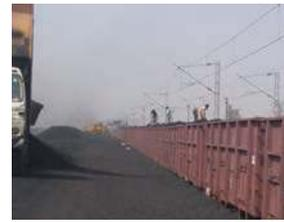
Figure 1. Filling rail cars with rubber tyre loaders.
