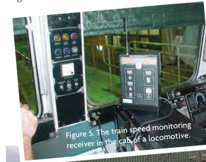
Figure 5. The train speed monitoring receiver in the cab of a locomotive.
