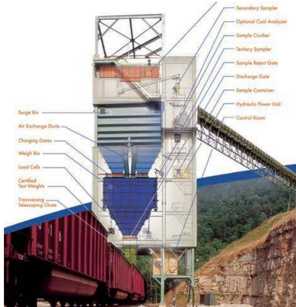
Figure 3. Batch weigh loadout system components.
