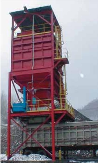
Figure 2. Volumetric loader.
