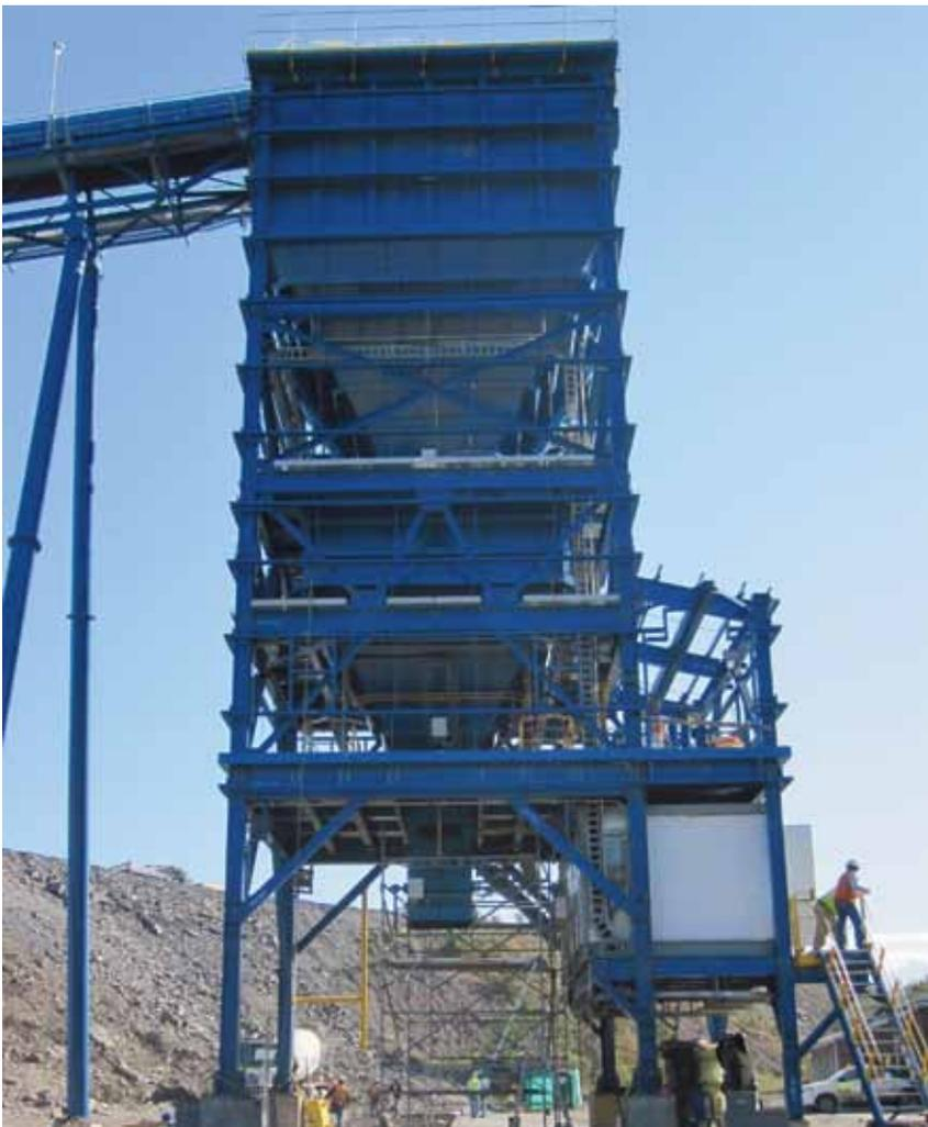
Figure 4. Pre-weigh loadout.
