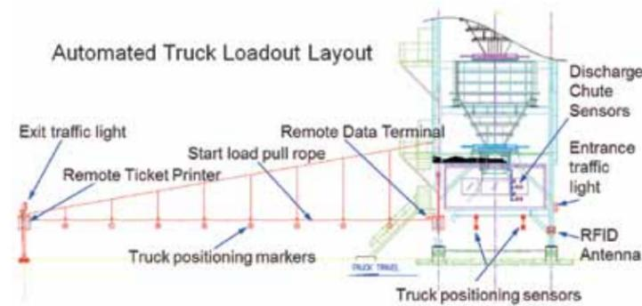
Figure 6. Unattended automated loadout.
